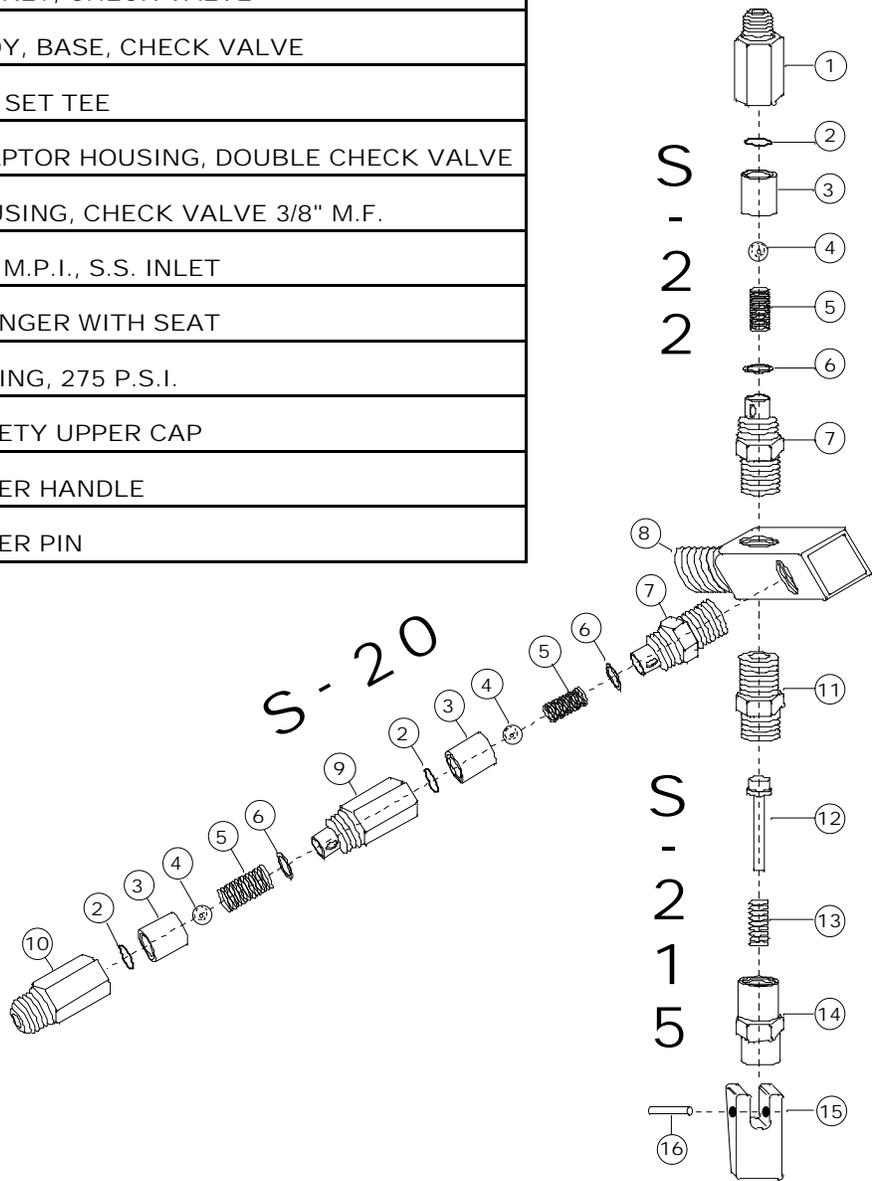
FIGURE 5-3. EXPLODED VIEW CHECK VALVES
