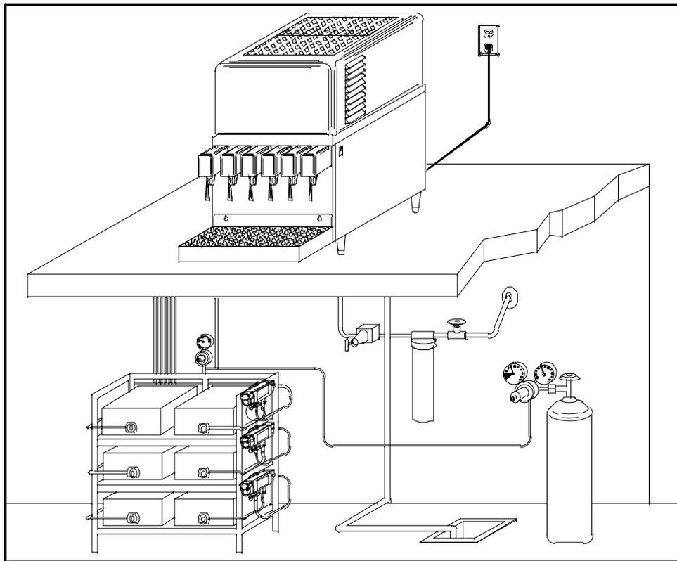
FIGURE 2-1. SAMPLE OF POSSIBLE INSTALLATION.
