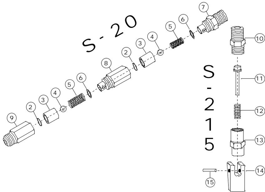
FIGURE 5-3. EXPLODED VIEW CHECK VALVES
