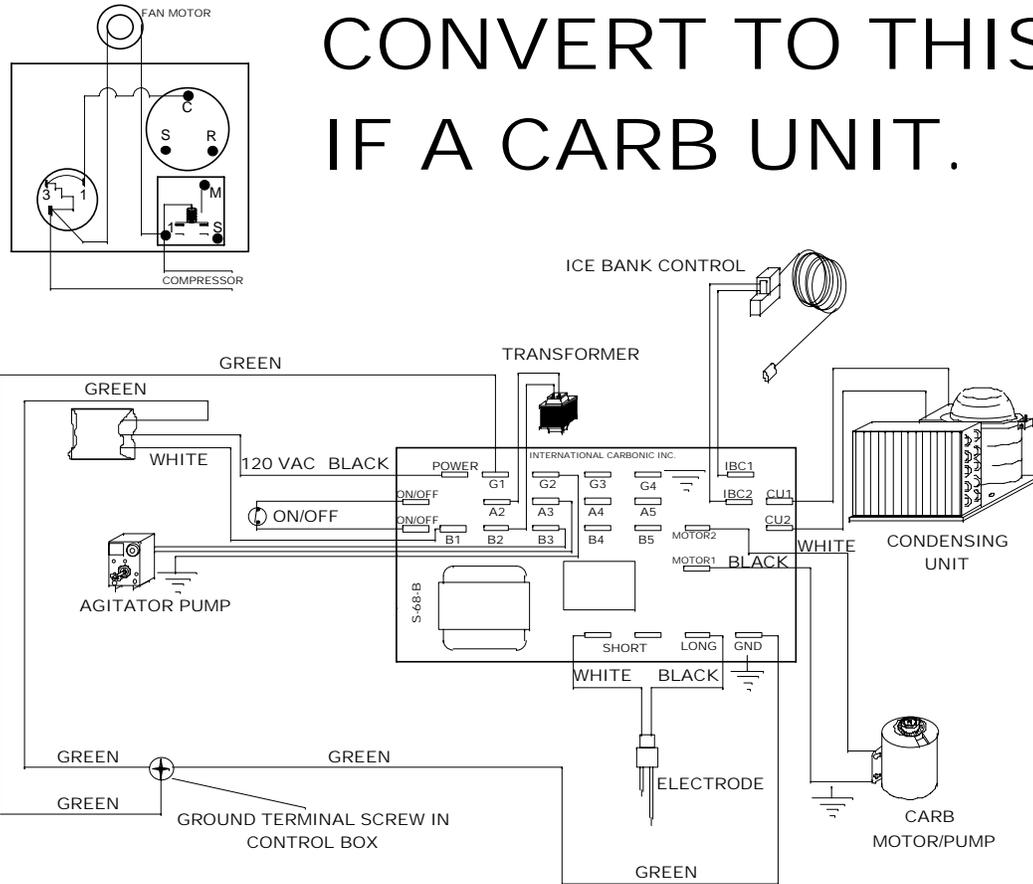
Note: Ground Terminals, Carbonator Tank
